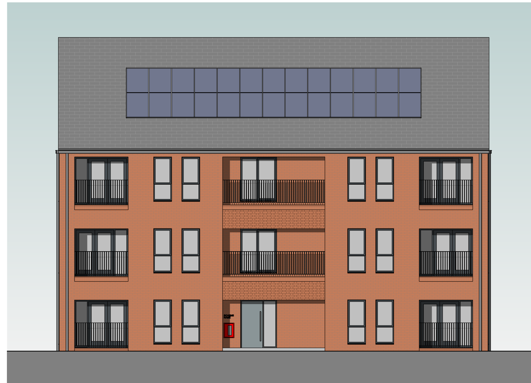
FRONT ELEVATION FACING COURTYARD PARKING 1:100
