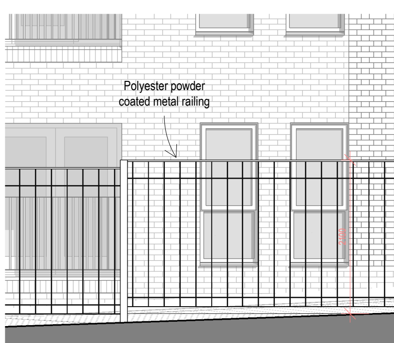
BOUNDARY TYPE A ELEVATION 1 : 50
